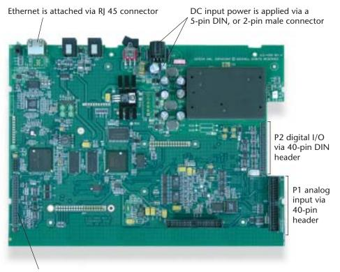
P3 frequency I/O, digital I/O and optional analog output via 40-pin header
